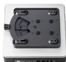
HP Quick Release attached to thin client
